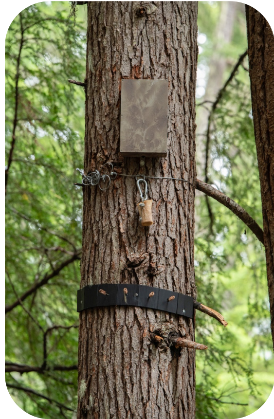
A scent dispenser, created by Robert Long, with accompanying hair brushes designed to attract martens and collect hair samples. Image Credit: Ben Wymer.
