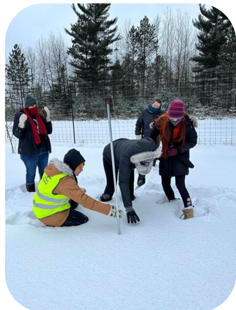
Below: FDLTCC students getting mid-winter snow water equivalent interval board measurements. Image Credit: Ariana Northbird.
